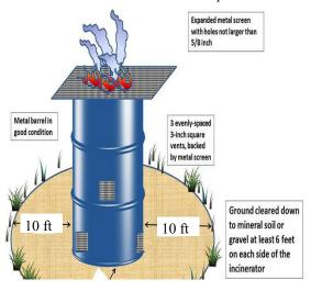
Make sure all openings are covered with screen to prevent embers from escaping and don't use a barrel with rust holes.
